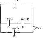
**23.** In the given network, find the charge on the capacitor.
